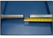
For ColorBar, the supplied Splice Connectors create a continuous run of bar therefore the bar ends should be no further than 1/8" apart. ColorBar butt joint connections can be made anywhere along the
